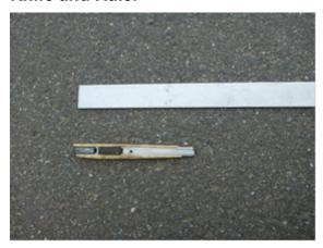
You cut fibreglass with the knife, and sometimes it is coated with epoxy. Therefore I have a knife with disposable blades that you can replace as needed. Use an aluminium ruler from the hardware store.
