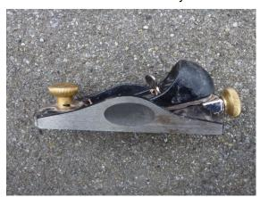
The plane blade is best sharpened on a fine abrasive paper sheets on a glass plate. I always use a few drops of oil when sharpening. Only a few strokes on an abrasive paper of 1200 grade, then use 2000 grade.
