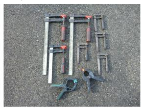
The spring clamps are optional. Unfortunately, epoxy coated parts are not held tight enough with the spring clamps to prevent slipping as parts cure. Therefore, you should use them together with clamps. Or secure the epoxied parts in addition with staples or nails to prevent slipping.
