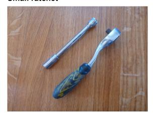
The small ratchet with extension and 7 mm socket is the only onboard tool you need. It is used to loosen and tighten the leeboard clutch mechanism. During the build, you are happy to have it for tightening the U-bolts at bow and stern from the inside of the boat.
