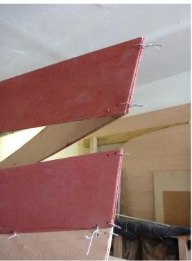
Wiring of plank 4 is much easier if you temporarily hold the plank with clamps to the frames:
