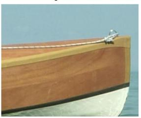
It is important that the new bow form is drawn first and looked at it from a few feet away. If the planks are once shortened, there is no turning back! In order to hold the bow straight, right and left planks must be processed exactly the same.
