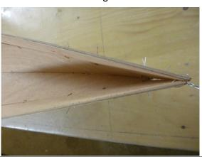
Arriving at the rear, first one plank, then the other, are sawed off flush to the skeg and filed, rasped, sandpaper rounded.
