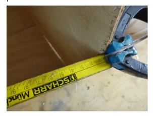
If the mould forces two adjacent planks apart, then it must be shifted somewhat to the middle. If there is, however, a gap between plank and bulkhead, then the bulkhead must be moved somewhat towards the end.
