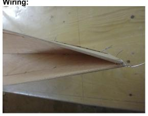
This bow is awry! The starboard side of the second plank has been tied in too over tight to the first plank. On the port side, the planks are not completely fair above each other:
