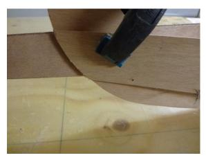
Then the planks are slightly chamfered inside with a rasp or with the planer:
