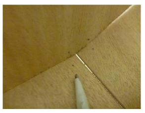
This is an example where the bulkhead forces the plank seam apart – so it sits a little too far forward. Two wires near the centreline and (later) two other wires in the gunwale are enough to hold the bulkheads in place. To avoid holes in the gunwale plank, the holes are drilled through the gunwale stringer only – and far enough apart that I can shift the bulkhead slightly if necessary.
