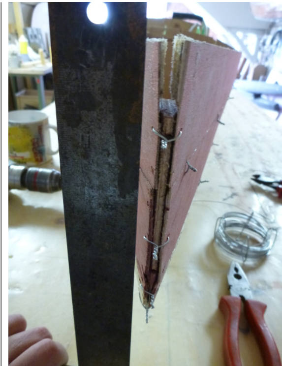
Unfortunately, the upper part of the bow is warped slightly to starboard:
